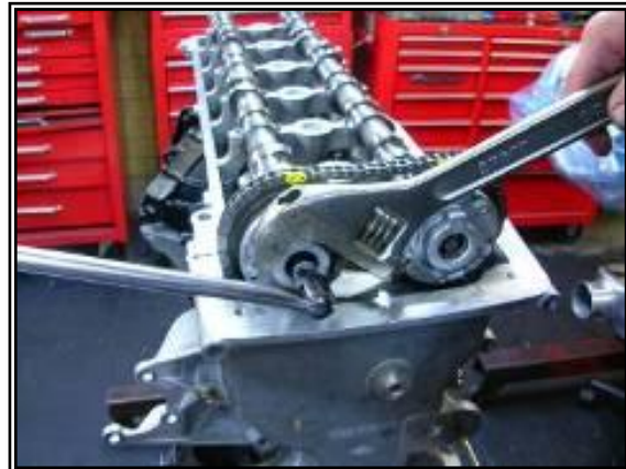
Figure 1 – Loosening the VCT bolts
