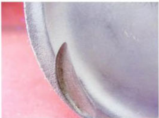
Figure 2: The #6 piston crown was typical of all the other pistons, and revealed dimpling of the squish bands and valve pockets that was characteristic of detonation.
