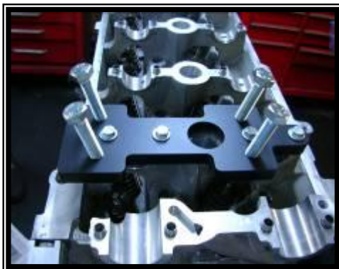
Figure 2 – installation of tool on head
