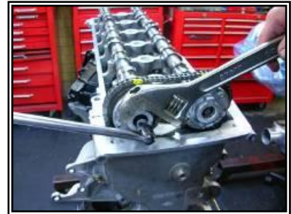
Figure 1 – Loosening VCT bolts
