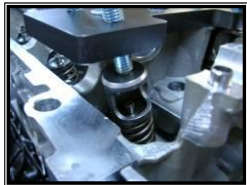
Figure 3 – fitment of collar and compressing of spring
