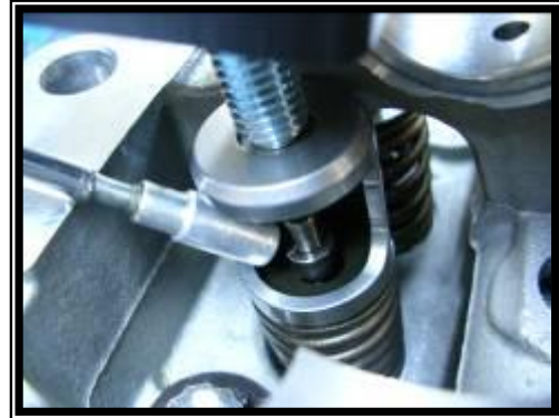
Figure 4 – removing the collets with the magnetic tool
