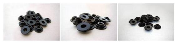
Machined from 4140 chrome moly bar stock, heat treated and black oxide coated for durability and appearance, they will fit stock valve springs and most aftermarket springs, including Atomic #306800, #306801 and #306802.
